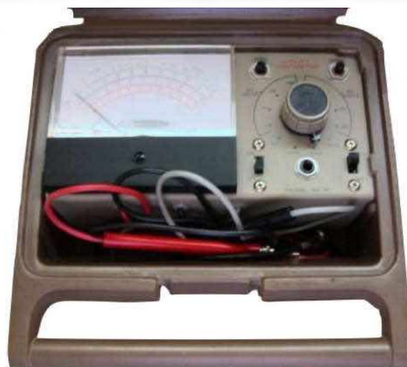
Figure 1: Later style IM-17 Solid State Utility Voltmeter
