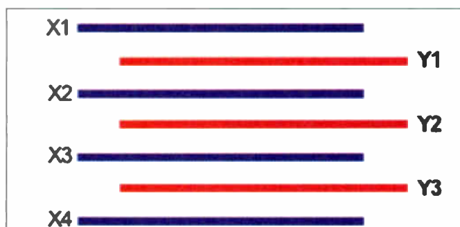
Fig. 9: ALiS panel line addressing.
